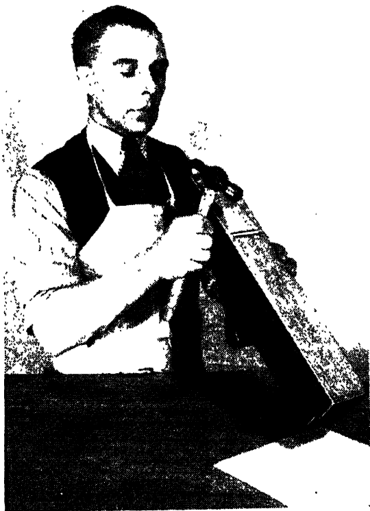
FIG. 14.—SETTING THE PLANE.
